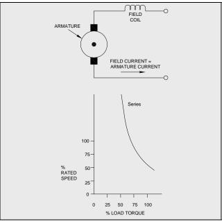
Figure 5-3: Series Field Motor
