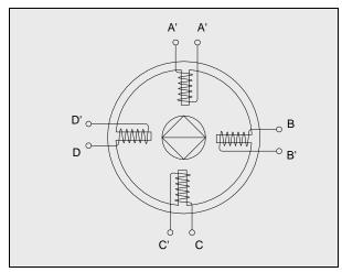
Figure 6-1: Electronically Commutated Motor (ECM)
