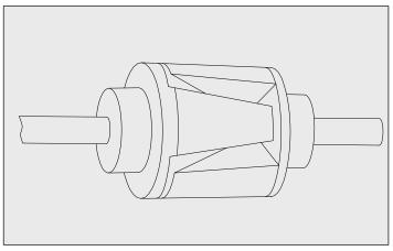
Figure 4-13: Non Excited Synchronous Motor Rotor
