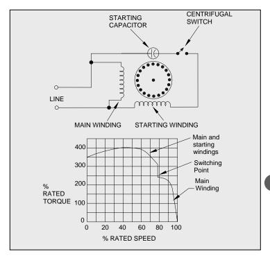
Figure 4-9: Capacitor Start Motor
