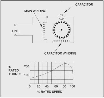
New furnace fan motors sometimes use capacitor run motors.
