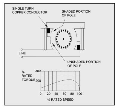
Figure 4-11: Shaded Pole Motor
