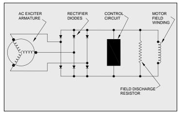
Figure 4-12: Exciter for Brushless Synchronous Motor
