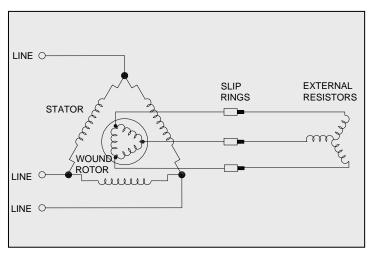
Figure 4-5: Wound Rotor Induction Motor
