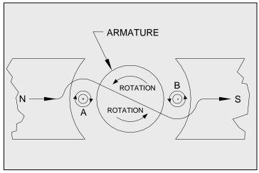
Figure 5-1: Torque Production in a DC Motor
