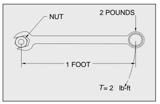
Figure 3-2: Torque Example
