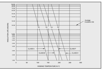
Figure 7-6: Insulation Life vs. Temperature
