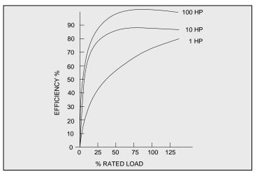
Figure 7-9: Typical Motor Efficiency vs. Load
