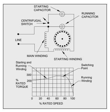
Figure 4-10: Capacitor Start – Capacitor Run Motor
