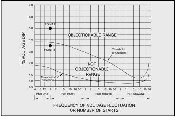
Figure 7-4: Voltage Flicker Curve - Example
