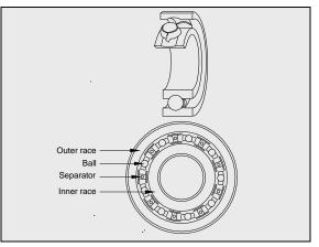
Figure 9-1: Antifriction Bearing
