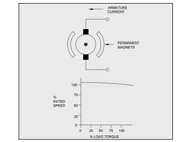
Figure 5-5: Permanent Magnet DC Motor
