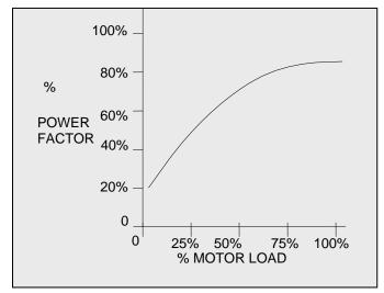
Figure 7-11: Typical Power Factor vs. Load<sup>2</sup>
