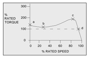
Figure 3-3: Typical Torque-Speed Graph
