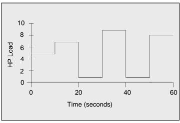
Figure 7-5: Repeating Duty Cycle Curve
