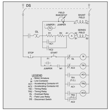
Figure 8-7: Example of a DC Motor Starter
