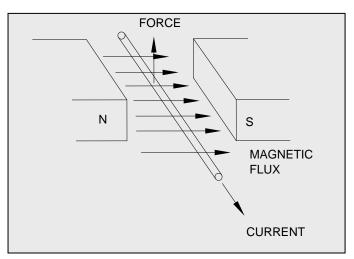
Figure 3-1: Force on a Conductor in a Magnetic Field
