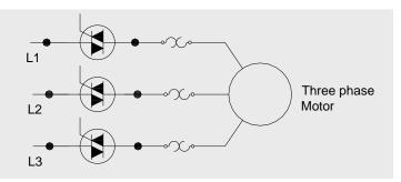
Figure 8-5: Solid State Starter (Simplified)
