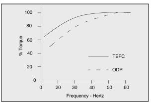
Figure 8-8: The Effect of Reduced Cooling on Torque Capability
