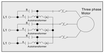
Figure 8-4: Autotransformer Starter
