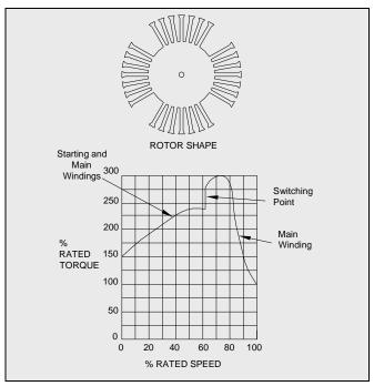
Figure 4-14: Single Phase Reluctance Motor
